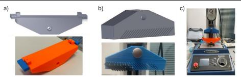
Figure 1 - a) Tool of fixation and rotation of the PCL fibres. b) Cutting tool. c) Multitest 2.5-dV machine equipped with the fixation, rotation, and cutting tools.
